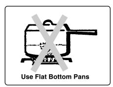
Use flat, heavy bottom pans that stay flat when heated for the best results. Avoid cookware that is warped, dented, ridged or thin. A warped or ridged pan receives the most heat at the points that contact the flame. This can result in burning or scorching of the food being prepared.
